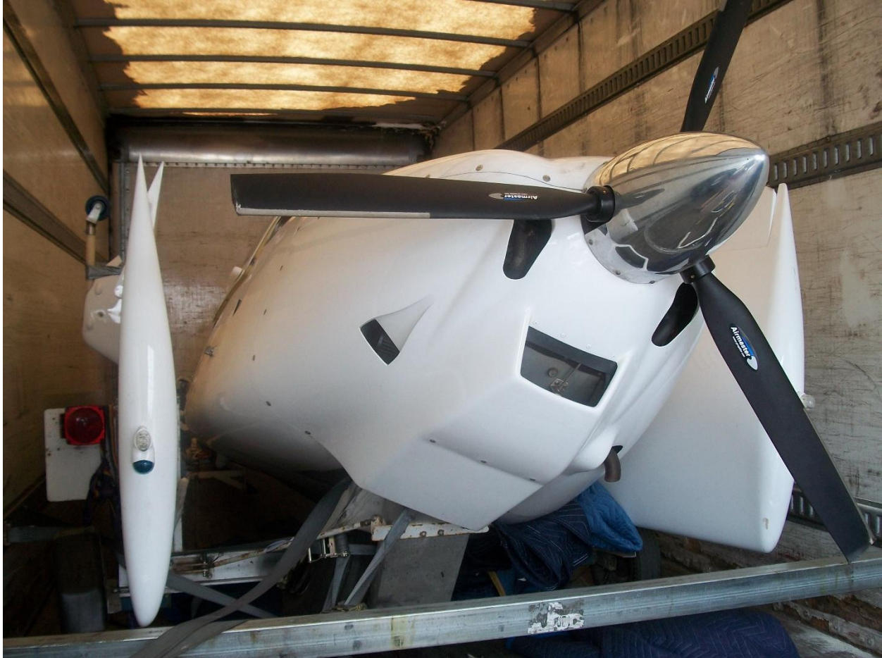
Failure to secure the Europa Mono to the trailer leads to a disaster on the road.
